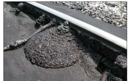
Flood-type wiper bar = clogged ports divert grease to the ONLY open lube port
