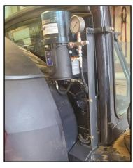
Each FLO system consists of a G-Mini® 12 VDC pump with built-in heater and 1L grease reservoir, SSV positive displacement grease metering valves, and fittings, tubing and hose with standard re-usable hydraulic hose ends and adapters. Space for attachments on compact equipment is at a premium. FLO technicians worked closely with the customer to custom fabricate the mounting brackets onsite, to mount the pump in a location where it wouldn't obstruct equipment operation.
