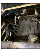
Remote Engine Shutdown Kit. Engine shutdown is especially useful in helping to limit damage from fires intensified by hydraulic fluids or fuel. The kit uses a pressure switch connected into the wiring for the engine fuel pump. Upon activation of the FSS, the pressure switch is energized, which electrically signals a power turn off to the fuel pump, stopping the flow of hydraulic fluid and fuel through the sprayer and resulting in the engine shutting down.
