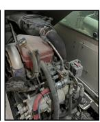
Remote Engine Shutdown Kit. Engine shutdown is especially useful in helping to limit damage from fires intensified by hydraulic fluids or fuel. The kit uses a pressure switch connected into the wiring for the engine fuel pump. Upon activation of the FSS, the pressure switch is energized, which electrically signals a power turn off to the fuel pump, stopping the flow of hydraulic fluid and fuel through the dumper and resulting in the engine shutting down.
