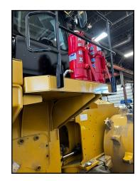
chemical agent part of the system rapidly cools super-heated temperatures and components, thus avoiding fire re-ignition.
