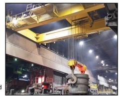
FLO for an Automatic Lubrication Solution to ensure the trolley hoist bearings stay properly lubricated. Employee health and safety was also a factor, given the height and location of the crane and difficulty involved to lube it.
