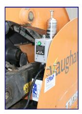
Before installing the SM Luber, they were manually greasing the skid steer. "It just didn't make sense from a maintenance stand-point. It cost too much time to have the guys stop and grab the grease gun; then the grease would run out; and it just wasn't getting the kind of grease it needed. It's a lot more efficient to have an automatic greaser. With Automatics it's on a timer so it greases a lot more efficiently."
