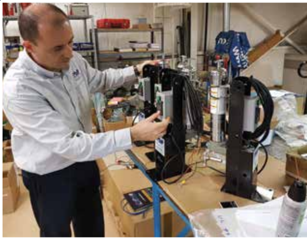
Flo's Gabriel Lopez demonstrates the Small Machine Luber, a compact yet powerful automatic grease system for compact equipment that is designed to use standard off-the-shelf industry grease cartridges.
