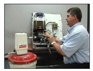
WARNING! – Even after you disconnect the air line, there is still pressure in the grease hose and the control valve, so always make sure to bleed that pressure back into the drum or another container.
