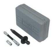
The Impact Fitting Cleaner is a time-saving alternative to fitting replacement and joint disassembly. Designed to eliminate downtime caused by dried blockages, the Impact Fitting Cleaner clears obstructions by allowing lightweight oil or solvents to enter the clog with a quick burst of pressure. It also cleans bearing and joint surfaces of hardened grease so that fresh grease can be applied.
