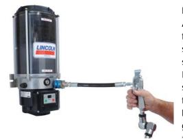
Lincoln has introduced its new ALS Fill Pump Kits for quickly filling automatic lubrication system reservoirs in lube truck, shop or plant applications. Developed for small- to mediumsized reservoirs, these kits feature Lincoln's high-volume PMV 25:1 pumps which deliver grease up to three times faster than similar 50:1 pumps.
