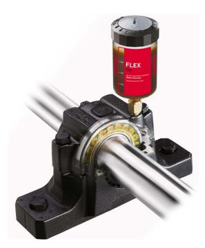
FLO Components is now offering the new perma FLEX, an ideal single-point lubrication system for all types of applications and industries. This gas generating unit produces the required pressure to continuously supply the lubrication points with fresh lubricant for the selected discharge period. And activation has never been easier - just turn the switch to the required discharge period (1 - 12 months) and perma FLEX is ready to go.
