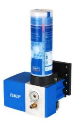
Developed to lubricate bearings and linear guides in small machines, this reliable pump includes an integrated pressure-relief valve that enables its use in single-line lubrication systems.
