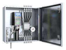
SKF has introduced the Lincoln electrically driven lubricator (EDL1). Utilizing progressive metering devices, the EDL1 allows you to have one centralized reservoir supplying several sectional lubrication systems or a large machine with different lubrication requirements at varying distances. This easy to use dosage and pressure-booster pump is
