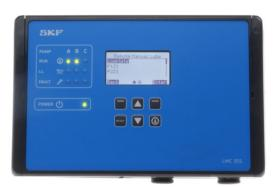
Designed for use with pumps that have no built-in controller, the LMC 301 combines all critical lubrication system management functions in a single package, simplifying system setup, operation, monitoring and maintenance.
