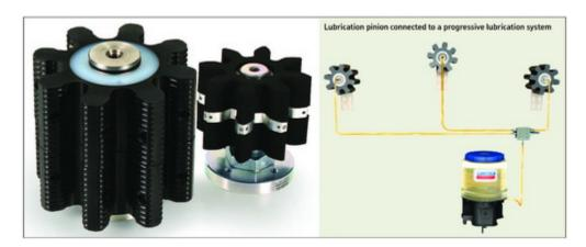
These pinions can be connected to an Automatic Lubrication System to provide the tooth flanks with the appropriate amount of lubricant. The lubrication pinions do not require pressurized air. Therefore, no spray mist contaminates the environment. In addition, NLGI grade 2 grease can be applied. When compared to manual lubrication, use of these pinions provides better quality lubrication, and reduces labor and the risk of accidents.
