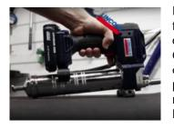
Debris and contamination is the #1 cause for failure of grease gun operation. In this video one such unit is evaluated and repaired. Cleaning and maintaining equipment is essential to reducing unwanted downtime. The process covered here takes only a few minutes and should help equipment last longer and stay in the field longer.
