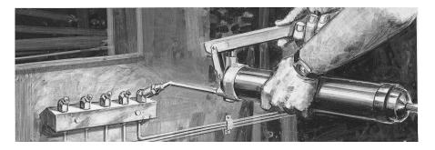
To set up a Remote Lube Fitting System, you remove the existing grease fittings at the bearings and replace them with tube fittings. Then run nylon hose or steel tube from the fittings to the manifold. Each line will have its own grease fitting on the manifold. This relatively simple and low-tech solution offers several benefits:
