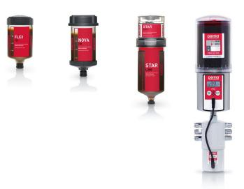
Single Point Lubricators (also referred to as drip feed lubricators or drip greasers) are a relatively inexpensive solution. Simply install the Lubricator either directly on the bearing or through a remote line, set the timer as applicable, record the scheduled time for replacement and there is one less lubrication point to worry about. Typical applications for these units include: electric motors, pumps, roller and slide bearings, chains, conveyors bearings and chains and open gears.
