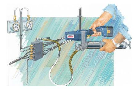
As an additional benefit, using the divider valve you only have to hook up the grease gun to a single grease fitting to service multiple points (instead of multiple fittings with the manifold).
