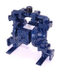
of Dual-inlet, Air-operated, Double-diaphragm (AODD) Pumps for continuous use in heavy-duty vehicle service and industrial applications, manufactured by Lincoln of St. Louis. Originally developed for antifreeze/water mixtures, the pumps dispense other light fluids compatible with Buna-N, aluminum and/or polypropylene.
