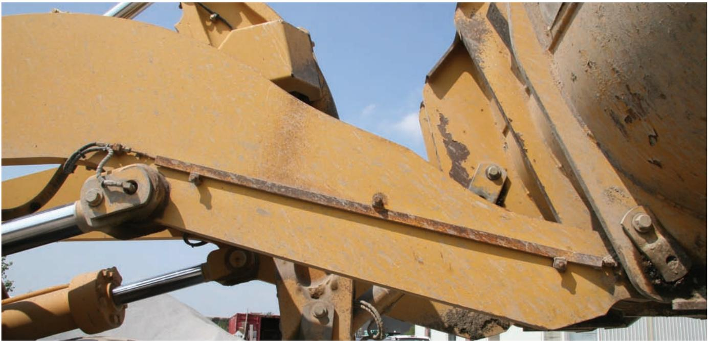
Supply lines are routed to recognize machine movement in order to minimize kinks or chafing and are protected in vulnerable areas such as loader arms. The manifolds incorporate grease nipples to enable manual or local greasing to be completed if necessary. Mussato is of the view that the system is a useful addition to all three pieces of equipment and delivers a noticeable improvement in component life compared to manual lubrication.
