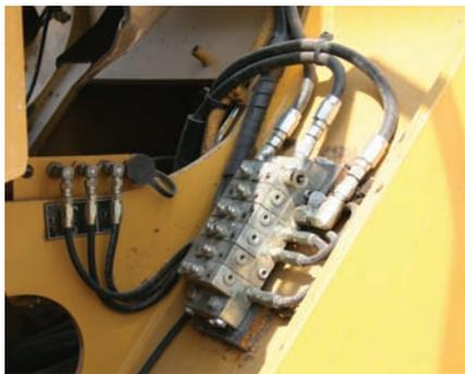
measured amount of grease at frequent intervals to each bearing covered by the system, based on pump timer settings and machine running time.
