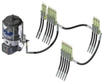
The nature of a parallel type system is such that only main-line pressure is monitored, so if any feed line or bearing is not taking lubricant, the remainder of the system will continue to function normally, but the lubricant-starved bearing may be lost.
