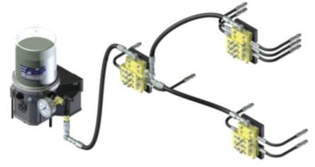
The nature of a single-line progressive system is such that if any line/bearing is not taking grease the entire system shuts down and there is (in a properly designed system) visual indication to the operator that there is a problem. This allows the operator an opportunity to take action before any damage occurs.
