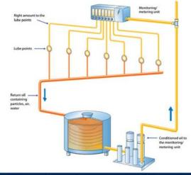
CircOil lube systems perform many functions, including filtering out wear particles.
