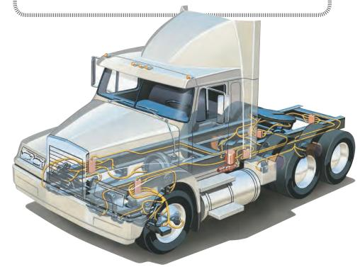
Operation begins when the controller/ timer sends a signal to the pump starting the lube cycle. The pump station automatically delivers lubricant through a supply line to multiple metering valves that then measure and dispense a predetermined amount of lubricant through feed lines, to the individual lubrication points.
